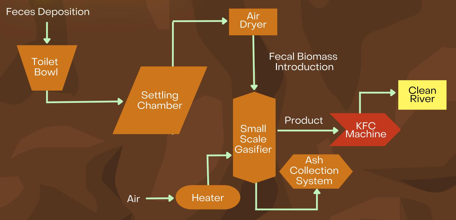
Figure 1. The operation of Project KFC with the flow process of the fecal biomass adopted from Cartmell et al. (2016)
